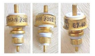
Miniature planar cermet triode designed to operate as low-power local oscillator in the C-band, up to 6000 MHz.
