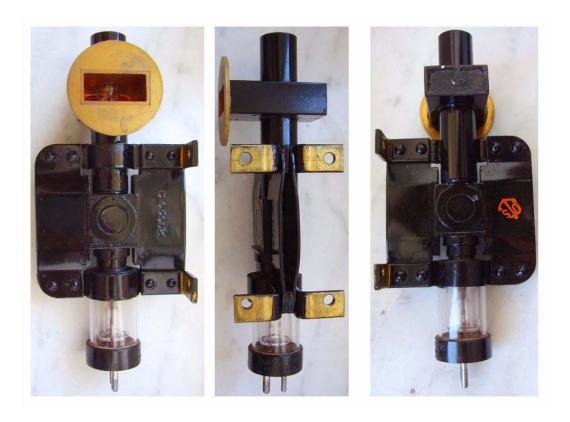
Fixed frequency, 9375MHz, magnetron capable of delivering 51 kW pulses. The 730A uses the same electrodes of 725A, with the flanged waveguide rotated 90 degrees. Bi-pin base.
