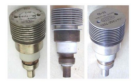
UHF planar pulse triode, ceramic version of the  $\underline{2C39A}$ . Also known as  $\underline{3CX100A5}$ , EIMAC.
