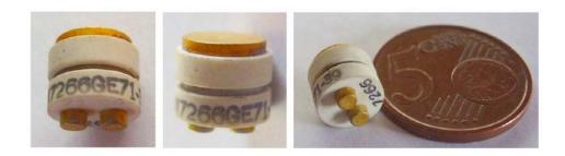
Very tiny cermet diode, capable of operation at frequencies as high as 7.5 GHz. 600 V PIV, 2 mA DC current, 10 mA peak. 6.3V at 0.215A heater. General Electric, August 3, 1959, record 2550.
