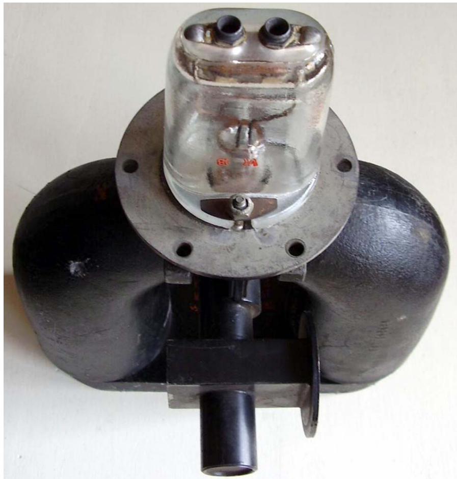
Photos of a 725A mounted in the polepieces of a 14 lbs. permanent magnet
