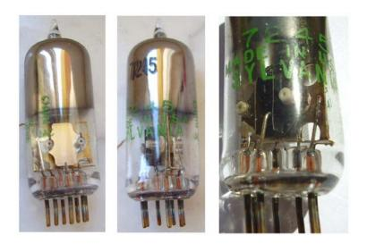
Stacked electrodes UHF triode designed by Sylvania as ruggedized version of 6J4. The family of stacked triodes with ceramic spacers, intended for highly automated production lines, started around the mid fifties with ceramic envelope prototypes, capable of operating at high temperatures. Later the same electrode assemblies went into production within glass envelopes and miniature bases. Here the article from <u>Electronics, August 1954</u>.
