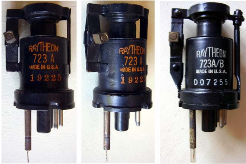
A sample of 723A made by Raytheon, left and middle, near an improved 723A/B to show the visible differences, Click on image to enlarge.
