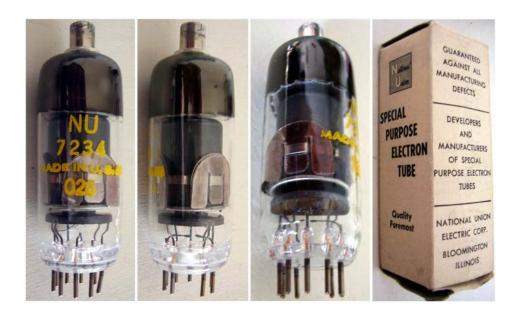
This pentode was designed as high-voltage regulator or control amplifier in power supply circuits operating from 3 to 8 kV. For its low capacitances, its high gain and its slew-rate it was also useful in high-voltage sweep circuits. In a T  $6\frac{1}{2}$  envelope, about 65 mm high, it was capable of 10 W anode power dissipation.
