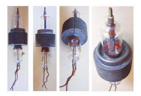
Forced-air cooled 'micropup' UHF transmitting triode. External copper anode with finned radiator, parrot-cage grid supported by the long rod through the top glass dome. Thoriated-tungsten spiral filament.
