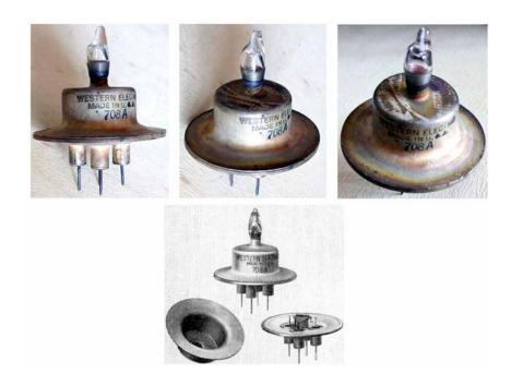
UHF grounded grid mixer triode for radar receivers. Flanged steel body with grid connected. Three coaxial feed-through pins for filament and anode from the bottom plate. The fourth pin, the grid, is connected to the metal shell. Top glass vacuum seal.
