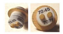
Ceramic-metal small-size high-gain planar triode.
