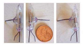
UHF subminiature diode mixer/detector. T2 body, plate pin out from the side, flying leads for the heater. 1.5 kV PIV, 10mA. 0.5A at 4.5V heater.
