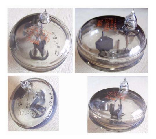
Doorknob shaped UHF transmitting triode, usable as oscillator, amplifier or mixer up to 1500MHz. 20W anode dissipation. 4.5A at 1.15V filament.
