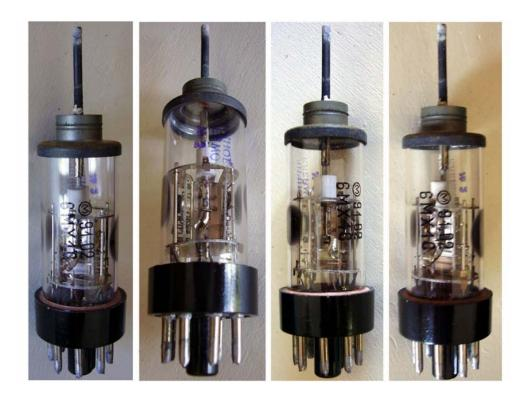
Mechanical displacement sensor. The two anodes are mechanically connected to the sensor rod which exits from envelope through a flexible diaphragm.
