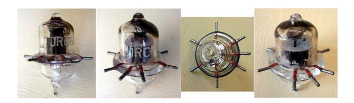
UHF 'acorn' triode intended as RF power amplifier or oscillator at frequencies up to 1200MHz. 2W max plate dissipation. Amplification factor 17.
