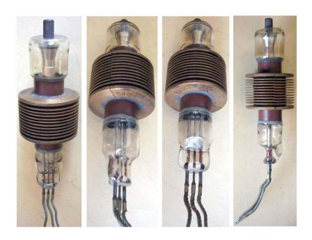
VHF transmitting or RF heating triode. Micropup shape with finned anode radiator. 600W anode dissipation; gain 30, 160MHz full ratings operation. Looks to be a ruggedized 8011.
