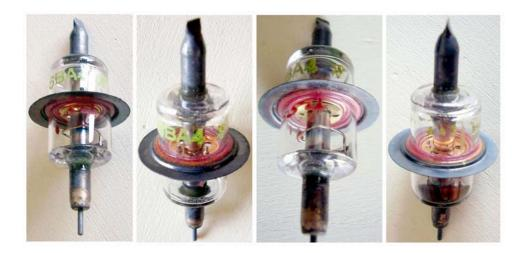
Planar disc seal triode, rocket style. Proposed by Sylvania as RF low noise front-end for UHF color television.
