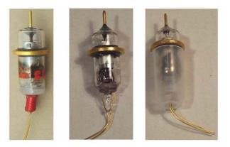
UHF signal diode intended for RF measuring probes.
