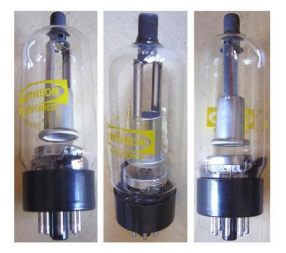
Beam-tetrode for use as high-voltage shunt regulator.
