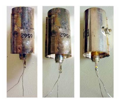
1680MHz oscillator module for radiosonde use, based upon a pencil triode.
