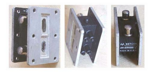
Dual integral cavity TR switch; 15 to 17 GHz, waveguide flange. 100 kW max peak power, 67 W max average. Two keep-alive caps, one for each switch.
