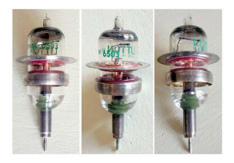
Rocket style planar triode. Ruggedized anode ring <u>2C37</u> for applications in critical environments. Superseded in the late eighties by cermet type <u>8980</u>.
