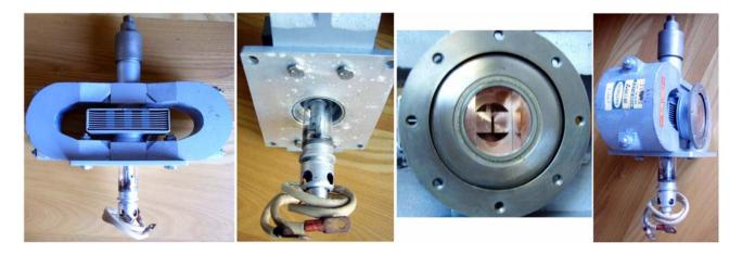
C-band tunable magnetron. Integral magnet, waveguide output, UG 148B/U flanged chocke. Forced air cooling required. Weight 25 lbs, about 12 kg. Raytheon
