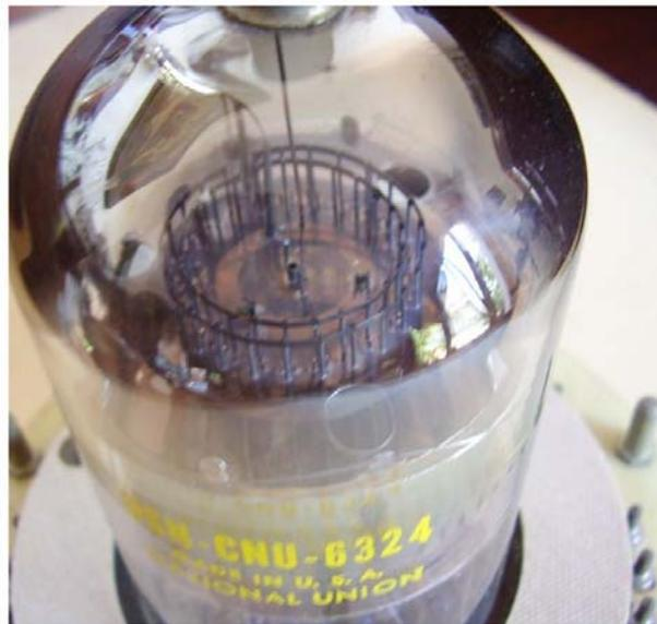
25 position beam switching tube, to be used in the transmission of multiplexed channels over a single carrier. The 25 grids are brought separately out, while anodes are all connected together. The tube has a special 33 pin base and a top cap. It requires an external magnetic field generated by a polyphase wound stator.
