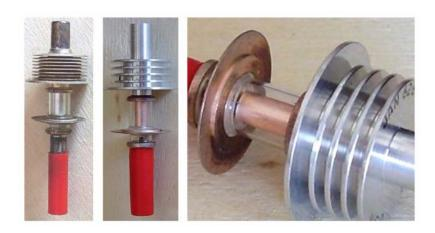
6263, left, and 6263A, center and right, are UHF power pencil triodes with integral radiator. Theese tubes were intended for use as RF amplifiers or oscillators in mobile or aircraft equipment at altitudes up to 60,000 feet. 6263A has improved radiator.
