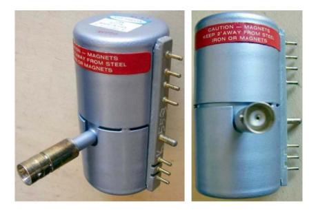
CW magnetron, integral magnet, BNC coaxial output. 220V DC at 30mA input, 1 W output at 4255 to 4370 MHz, frequency modulable within 2% by a voice-coil actuated tuner. Intended for radio-altimeter applications.
