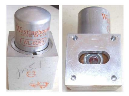
X-band, fixed frequency vacuum cavity. Flanged waveguide connections.
