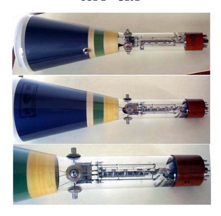
Circular screen 5" CRT. Electrostatic focus and deflection, undecal base.
