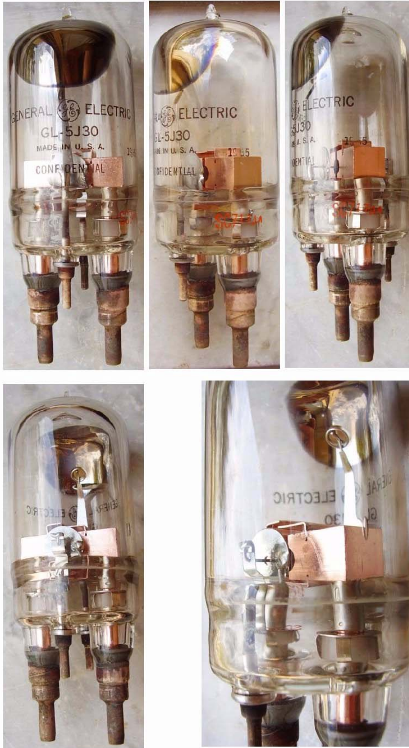
Photos of a General Electric GL-5J30. This magnetron was classified as ‘Confidential’, as etched on the glass.
