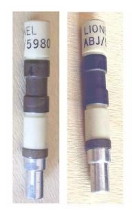
Gamma counter tube, cartridge shape.
