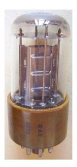
Tungsten filament operated around 4.4 Volts at 1.75 Ampere. 1.5 mA DC anode current at 90 V.
