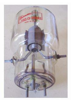
All-glass VHF power triode. Dual grid terminals out from side. Ruggedized design intended for RF heating or for VHF transmission applications.
