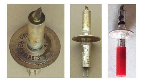
High-mu pencil triode usable as grounded-grid amplifier up to 1000MHz or as CW oscillator or frequency multiplier up to 1700MHz with full input or up to 3000MHz with reduced ratings. It was designed for operating in airborne or mobile equipment at altitudes as high as 60,000 feet.
