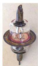
UHF planar triode intended for applications as CW amplifier or frequency multiplier in the range from 1 to 3 GHz. Proposed as RF front-end in television UHF tuners as in <u>Electronics</u>, October 1951.
