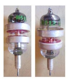
UHF triode with folded anode and grid rings. Can be used as amplifier or oscillator up to 3.3 GHz.
