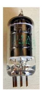
Miniature pentagrid converter, designed for reliable use in military or airborne equipment even in conditions of intermittent operation. Ruggedized version of 6BE6. 5000 minimum on-off cycles.
