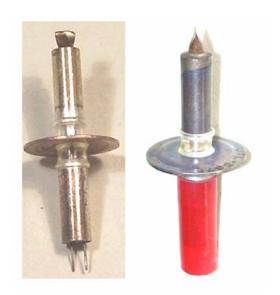
Pencil-type medium-mu triode usable as power amplifier or oscillator in coaxial resonators up to 3000 MHz.
