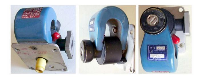
No info available on this Litton tunable magnetron. The waveguide flange size suggests an operating frequency around the X-band. Integral magnet.
