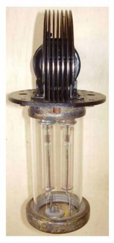
External magnet, coaxial output high-power pulsed magnetron. Forced air cooling required.
