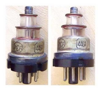
UHF planar, lighthouse shaped, triode. 446 can be considered the first lighthouse tube in production, followed by A and B versions and then by the <u>2C40</u>. It was used as UHF amplifier or mixer. As mixer it operated with noise figure better than that of crystal diodes up to about 1GHz. As amplifiers it operated up to about 3GHz.
