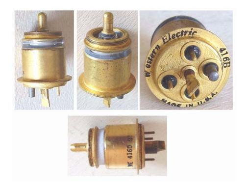
Planar triode, gold plated body; top pin to anode, threaded grid ring, four pin base. Glass spacers in the early versions, became ceramic in the late D version of the bottom picture. The 416B was registered as 6280. Characteristics improved in the years.
