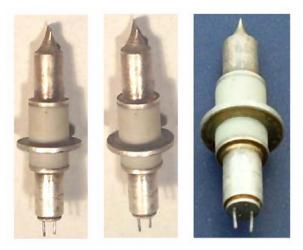
Cermet pencil triode, capable of operation up to 4GHz. Intended for use in navigation transponders. RCA proprietary code.
