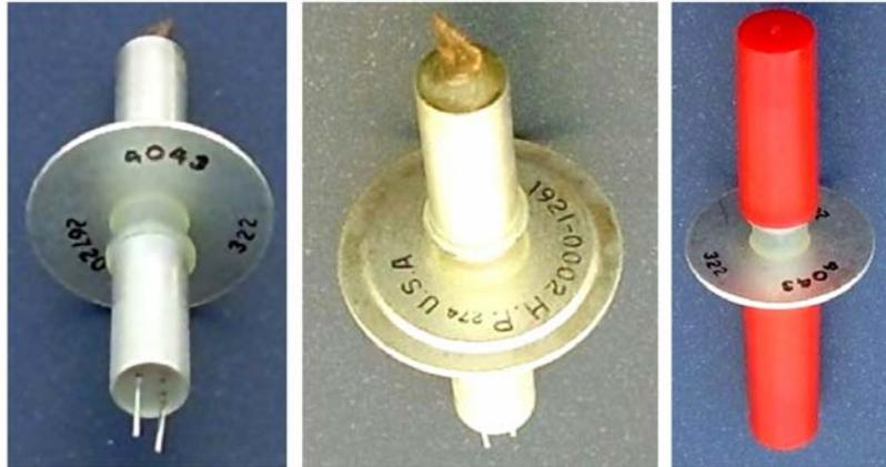
VHF pencil oscillator, capable of delivering 5 W RF output power at 500 MHz.
