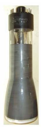
3" CRT with central deflection electrode for J-type indicators. Electrostatic focus and deflection, diheptal base. 4 kV accelerating voltage. 6.3 V at 600 mA heater.
