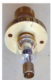
UHF transmitting triode rated for pulsed operation. Evolution of <u>3C27</u>, rated for higher duty cycle; integral grid radiator added. Some production lots of 3C27 were uprated by the factory to 3C27B, adding the grid radiator and a 'B' to the code, as in the sample above. Samples of both types can be seen in the <u>3C27</u> card.
