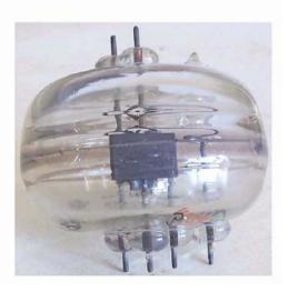
UHF triode, 50W anode dissipation, mu 6. Oscillates up to 900MHz. Grid and plate are supported by wires that run straight through the tube envelope: this geometry made it possible to mount the tube itself at the center of half-wave resonating lines. See also the article by A.L. Samuel, BSTJ vol. 26, issue 4 on 'A Negative-Grid Triode Oscillator and Amplifier for Ultra-High Frequencies'
