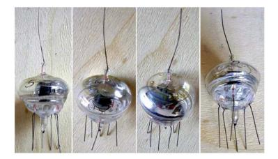
RF VHF pentode, member of a pre-war VHF family developed by Western Electric, family also including based types. Small 'mushroom' shape to keep leads as short as possible. During WWII these tubes evolved into miniature types, as the popular 6AK5.
