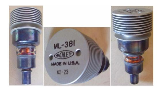
381 is a planar triode very similar to the industry standard <u>7289</u>. Oil-can shape, glass spacers. Intended for use as pulsed oscillator, frequency multiplier or class C amplifier in transmitting services up to 3.000MHz.
