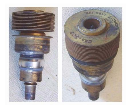
Planar UHF power diode. Intended for use as modulation clipper or frequency multiplier in cavity-type circuits at frequencies up to 1500MHz. Used in TR switches and VOR antenna systems.
