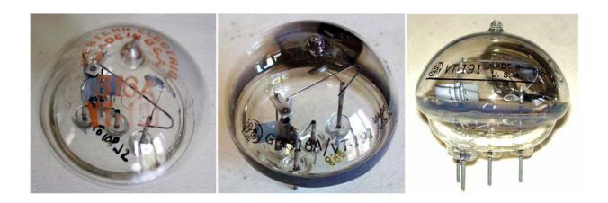
This odd shaped tube was introduced around 1936 by Western Electric as UHF power amplifier or oscillator. It was one of the few UHF tubes available before WWII, originating more powerful variants in the U.S. Also used in the very early British airborne radar prototypes and in Germany, where it gave origin to other variants by GEMA. All-glass body, closely spaced electrodes supported by short rods just over the base. A spring loop from the top keeps the tiny filamentary cathode in tension.
